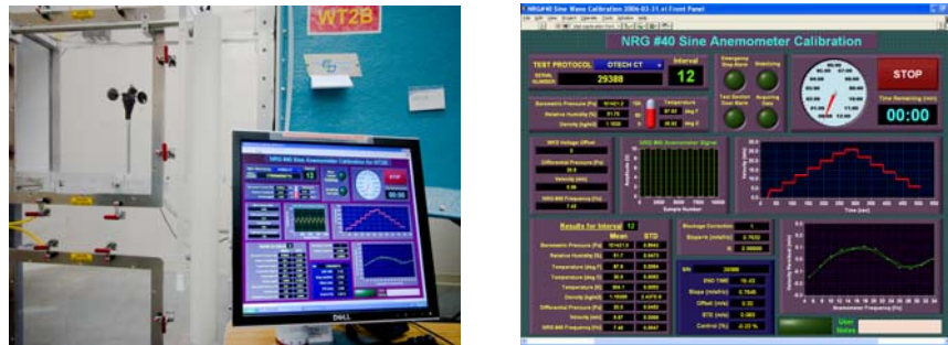
Figure 8: Calibration testing using LabVIEW wind tunnel control system and data acquisition.
